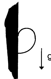
Fig. 6. Schematic of bubble adhering on a cavity in a vertical wall.
